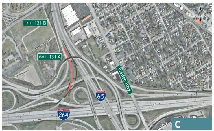
This would include reconfiguring the I-65 southbound exits to I-264 westbound and I-264 eastbound by separating the I-264 westbound exit from Exit 131 B and joining with the I-264 eastbound exit just north of its existing location. This would result in two exits: 131 B to the Fair/Expo Center; 131 A to I-264 westbound and I-264 eastbound. This improvement strategy can be done in conjunction with Improvement Strategy B.
