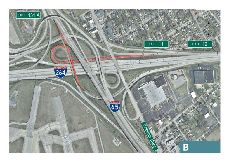
This would include improving the radius of the loop ramp from I-264 westbound to I-65 southbound and moving the traffic using this ramp from Exit 12 (I-65 / KY 61) to Exit 11 (Crittenden Dr.). The widened loop ramp would become an added lane of traffic to I-65 southbound just north of the bridge over I-264, and the I-264 westbound to I-65 southbound loop ramp bridge could be used by the I-65 southbound to I-264 eastbound ramp to improve sight distance.
