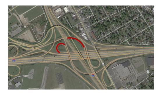
This would involve placement of a roughened pavement surface by either grinding pavement or installing a new surface treatment. Work would also include installing diagonal pavement markings along the shoulders of the curve of the ramps to prevent roadway departures and give drivers a visual cue to slow down. The high-friction surface treatment increases friction between the pavement and vehicle tires.
