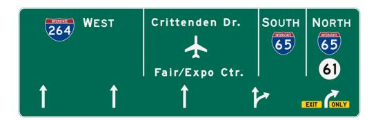
This would include installing new guide signage throughout the interchange to help drivers identify their desired destination. Signs would incorporate improved messaging, high-visibility retroreflective sheeting, symbols for popular destinations like the airport, consistent designations for exit only lanes and overhead arrow-per-lane signage where possible. Guide signage helps drivers navigate the interchange and can reduce unnecessary or last-minute lane changes.
